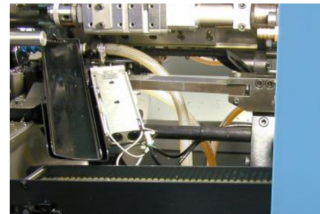
Part collector and Part conveyor
