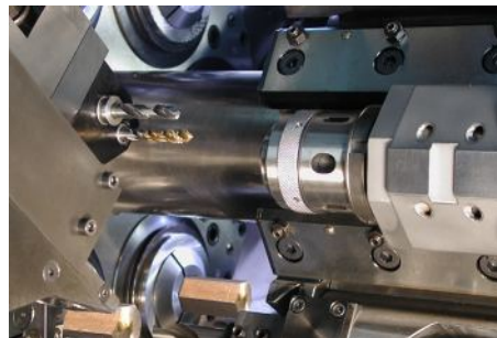
Synchronized pickup with additional cross slide for back working operations
