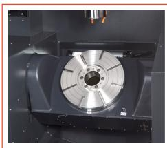
The flexible and wide tilting range offers the maximum Z axis distance for cutting application.
